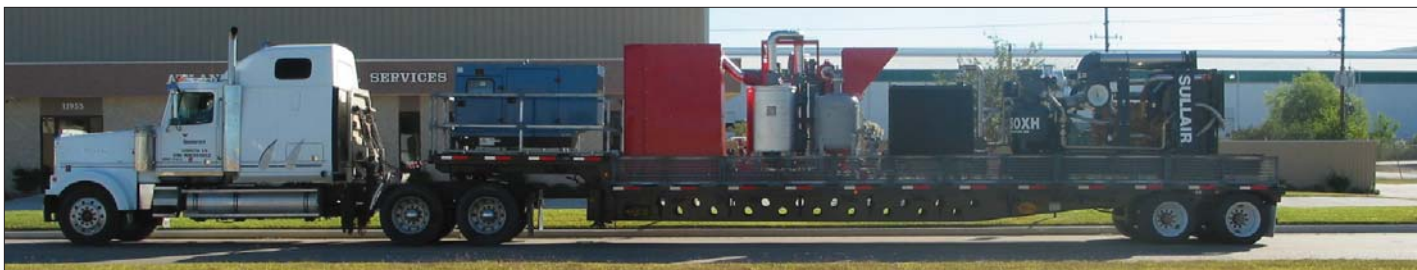
IGS systems built to specification for companies serving oil and gas operations can be mounted on a trailer in order to facilitate transporting them to wells.
